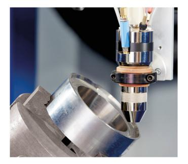
Subject to the required welding task and powder material, various electrode diameters, powder and plasma nozzles are available. Various torch designs with coaxial ring and 2 or 4 boreholes can be selected for the individual welding task.
