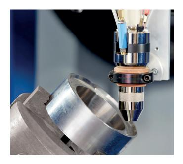
Subject to the required welding task and powder material, various electrode diameters, powder and plasma nozzles are available. Various torch designs with coaxial ring and 2 or 4 boreholes can be selected for the individual welding task.
